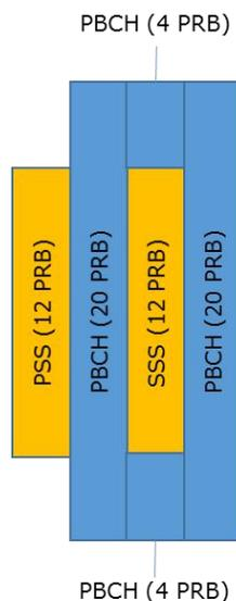
**Figure 5-2 Illustration of SS/PBCH block mapping**
