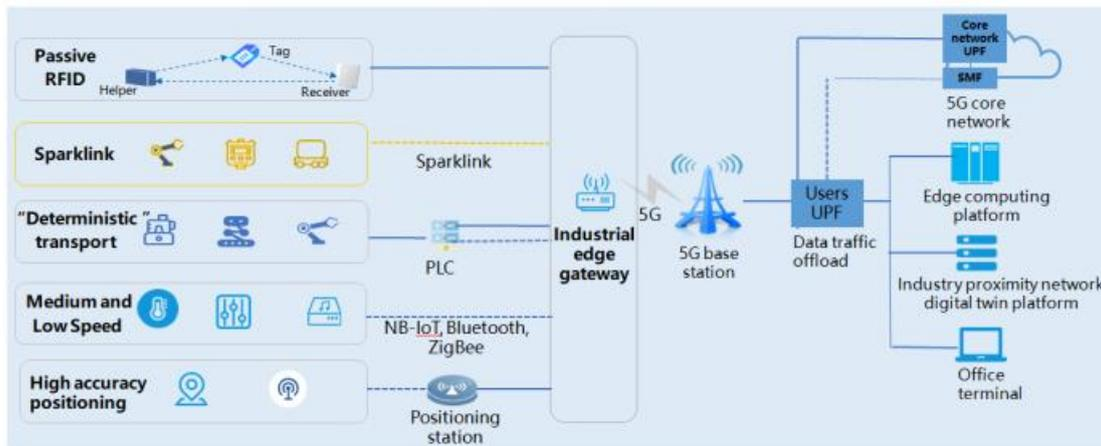
Figure 8. Overall architecture of 5G converged industrial proximity network
