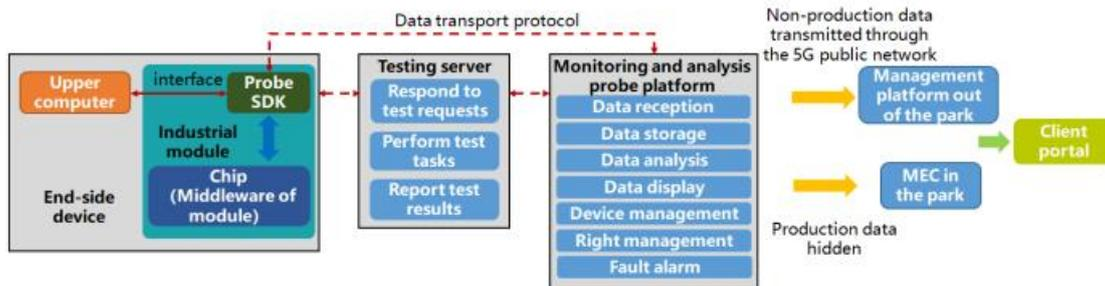
Figure 3. Architecture diagram of 5G end-side service quality probe system
