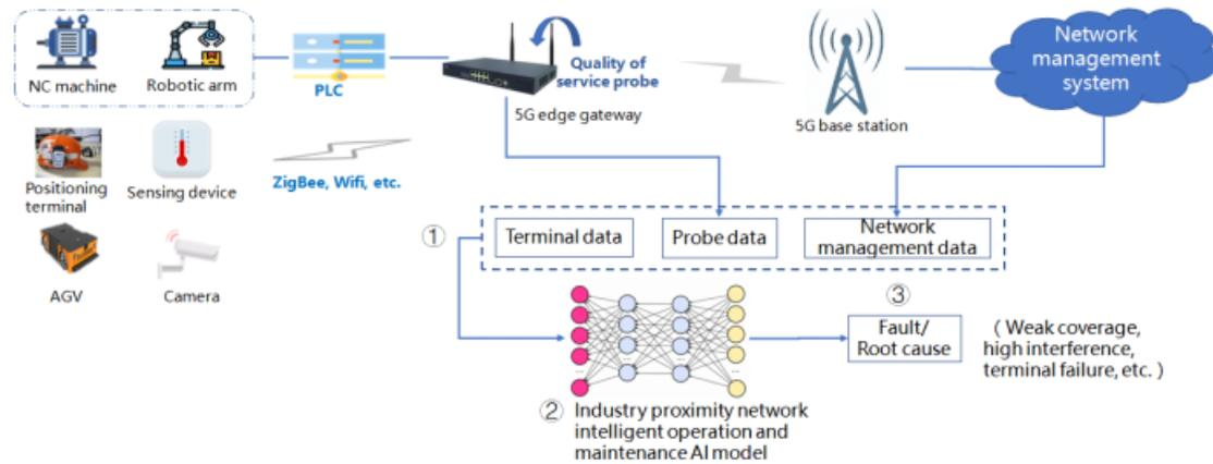
Figure 4. Intelligent O&M framework for industry proximity networks
