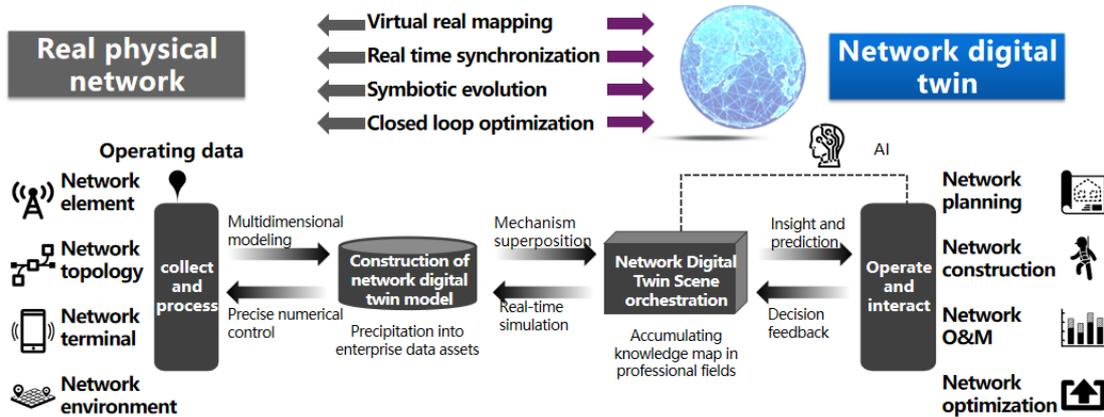
Figure 1. The principle and connotation of network digital twin
