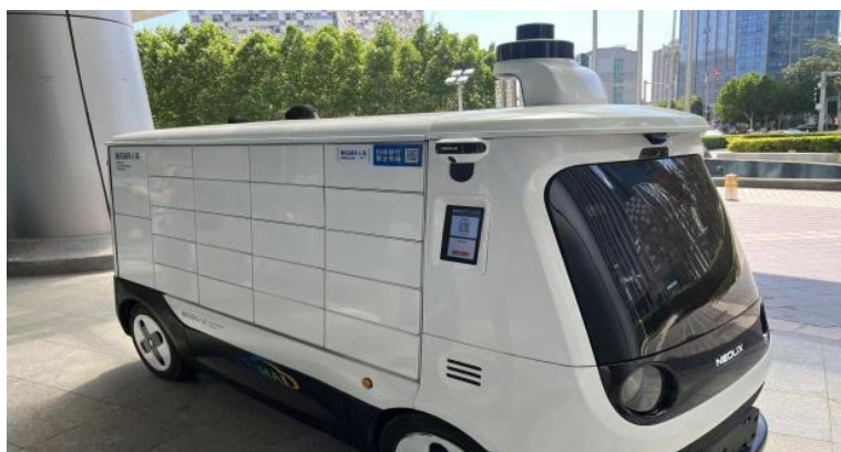
Figure 13 5G-enabled unmanned distribution logistics vehicle
